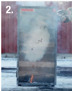
2. Once the battery ignited, the HDC cable reacted, activating the MAUS unit mounted at the top of the cabinet.
