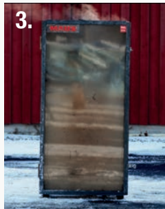
3. The active aerosol fills the space and suppresses the fire. The temperature drops to 104°F (40°C) within a few seconds.
