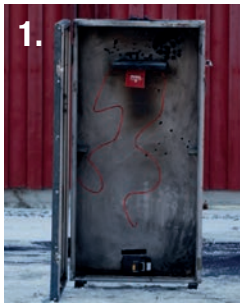
1. A lithium battery was placed at the bottom of the cabinet and the MAUS unit(s) were placed at the top of the cabinet.
