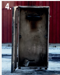
4. After 5 minutes, it was safe to open the cabinet and allow the non-toxic potassium aerosol to dissipate.
